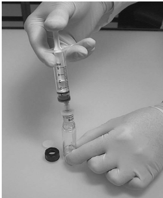
Fig. 6. Filtration of the reaction mixture through a silica plug into a standard vial.
